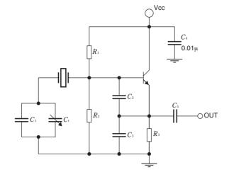
Select each circuit constant so that the adjustment ranges of upper and lower frequencies of this circuit are even on the basis of the frequency of a single crystal unit measured using a specified load capacity, and that the margin of  $\pm 8$  to  $10 \times 10^{-6}$  of the room temperature deviation of the crystal unit can be reserved.
