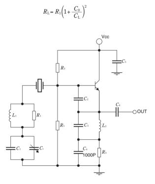
To prevent decrease in the negative resistance, connect the crystal unit to the base of the transistor as in the fundamental mode crystal oscillation circuit. To use the crystal circuit for both oscillation and multiplication, connect a parallel resonance circuit having multiplication frequency as resonance frequency to the collector of the transistor.
